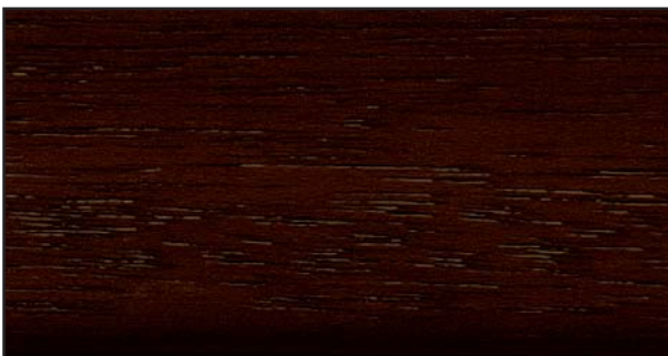
15 Species of wood: meranti Load group: B7/III-E Induline SW-900 Induline GW-360 Induline LW-700/40 clear wenge nut wood
