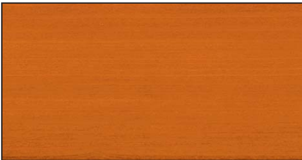
4 Species of wood: spruce Induline SW-900 clear Load group: Induline GW-360 teak B3/II-E Induline LW-700/40 cherry
